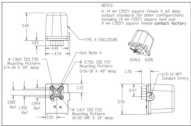
**Note:** Minimum height clearance for mounting: 7.43 in (18.87 cm)
