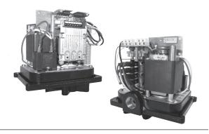
The MicroTorque actuator can be configured to accept 4-20mA, 1-5V, 0-5V, 0-10V, or a digital input signal. Two standard limit switches are preconfigured at the factory for 90° rotation. The stroke is field-adjustable from 30° to 270°. The **Polarity Detection feature** automatically determines which motor winding to control based on where the open and closed positions are set; this feature also eliminates the need to rewire the unit for direct or reverse acting applications.
